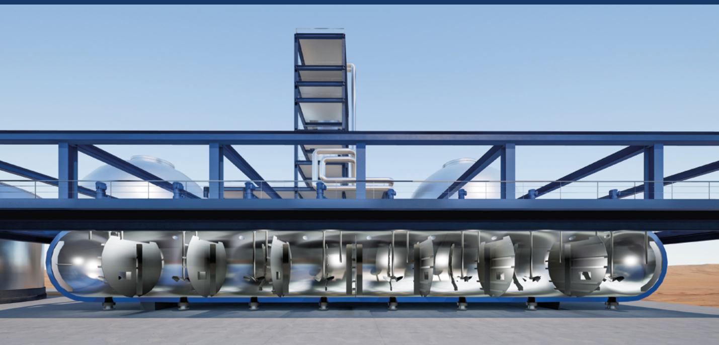
50 m long HPAL autoclave with eight compartments, equipped with EKATO EPAL-R impellers
