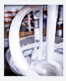
UNIMIX System: EKATO PARAVISC impeller with S-JET/V homogenizer (10.000 Liter unit)
