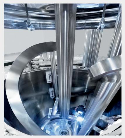
PARAVISC with flexible scrapers for improved heat transfer
