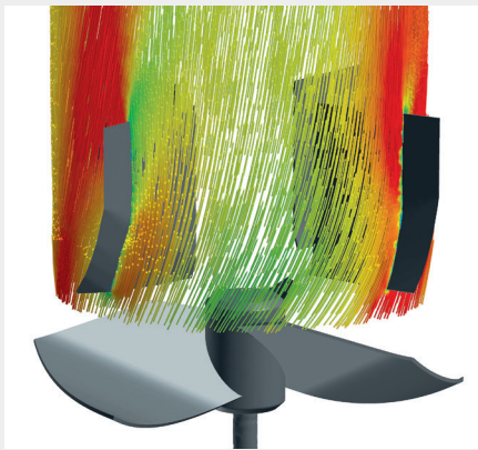
Well-balanced, low-shear flow field provides smallest possible strain on particles
